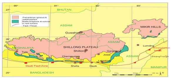
Figure 2: Regional geological map of Meghalaya showing main structures and Shella Limestone Occurrance. Based in part on Geological Survey of India (1981 & 2009)
